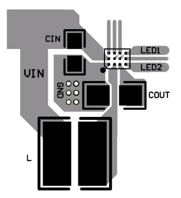
Figure 10. CSP Recommended PCB Layout
