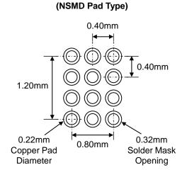
\* Dimensions are in millimeters.
