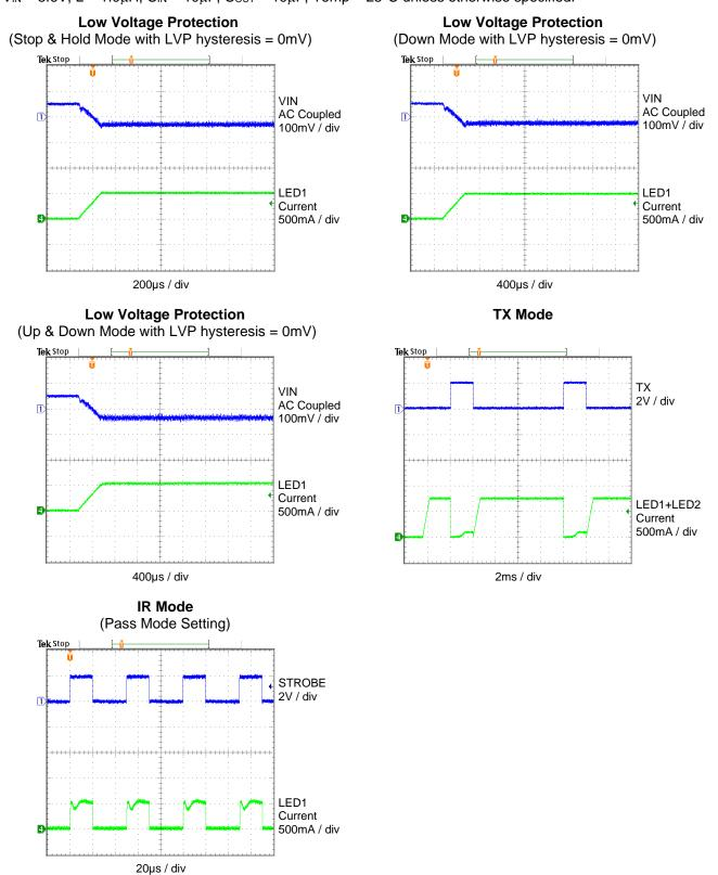
$V_{IN} = 3.6V$ , L = 1.0 $\mu$ H, C<sub>IN</sub> = 10 $\mu$ F, C<sub>OUT</sub> = 10 $\mu$ F, Temp = 25°C unless otherwise specified.
