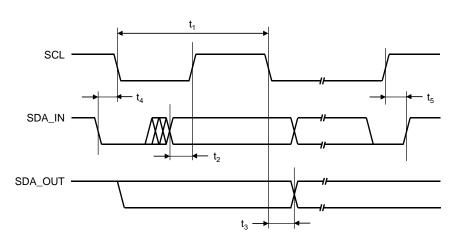
Figure 1. I<sup>2</sup>C Compatible Interface Timing
