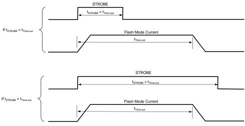
Figure 5. Flash Mode Current Controlled by STROBE (Edge Triggered)
