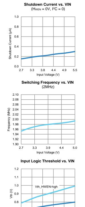
$V_{IN} = 3.6V$ , L = 1.0 $\mu$ H, C<sub>IN</sub> = 10 $\mu$ F, C<sub>OUT</sub> = 10 $\mu$ F, Temp = 25°C unless otherwise specified.
