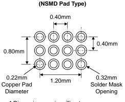
\* Dimensions are in millimeters.
