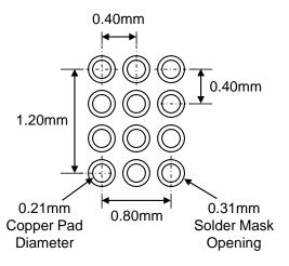
\* Dimensions are in millimeters.
