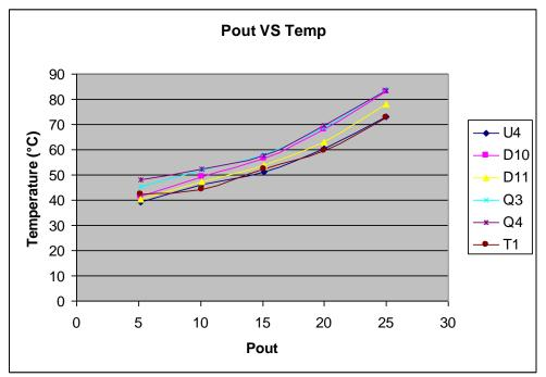
Figure 2: Component Temperatures within the AS1138 System
